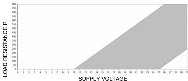
The diagram shows the optimum ratio between load and power supply for transmitters with 4...20mA output. For correct function, use a combination of load resistance and voltage that falls within the shaded area
