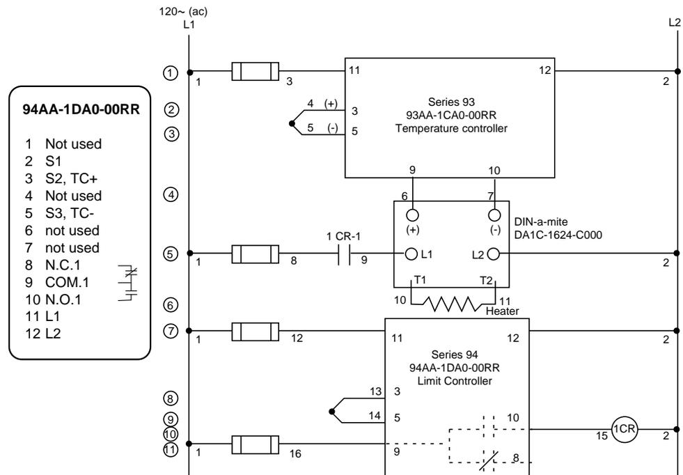
Figure 2.7 - System wiring example.
