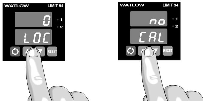
Figure A.3 - Entering the Calibration Menu.
