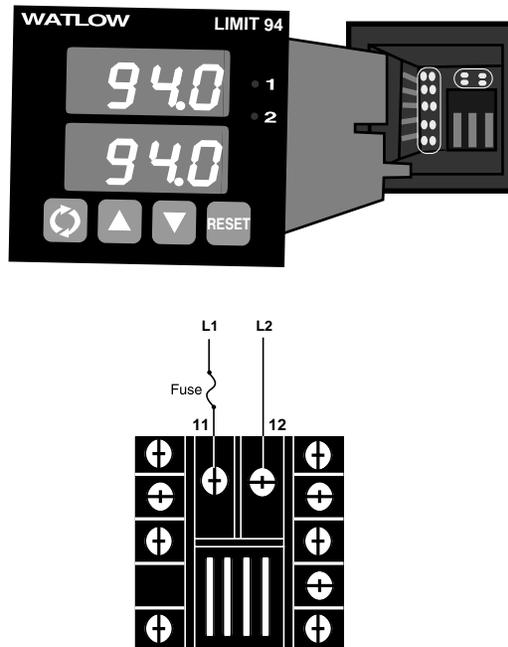
Figure 2.3 – Power wiring.
